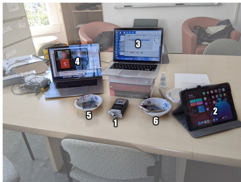
Figure 2: Phase 1 recording setup. (1) Zoom H4n; (2) ipad; (3) computer with internal microphone; (4) computer with external headset microphone; (5) android phone; (6) iphone. See supplementary materials for specifications
